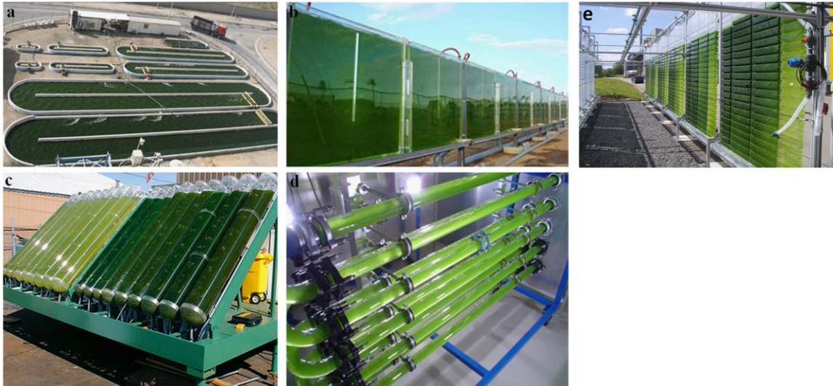
Figure 1.12 Large-scale PBRs (a) raceway pond, (b) flat-plate PBRs, (c) tubular type PBRs, (d) horizontal type PBRs and (e) Vertical column type PBRs [72]. Reprinted with permission from Elsevier.
