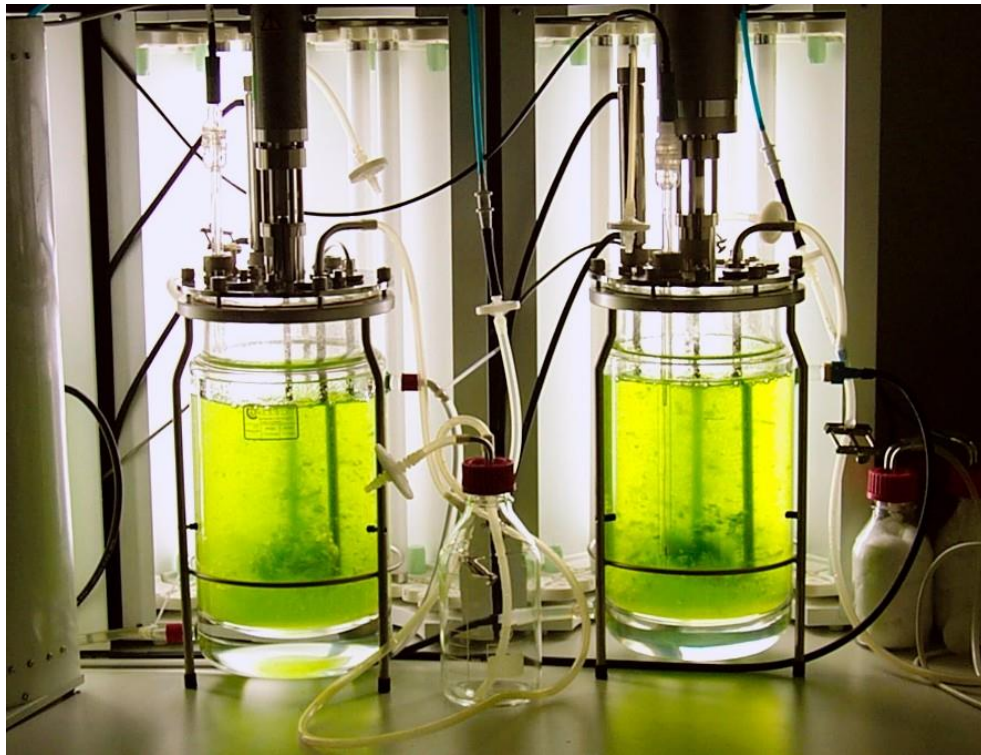
Figure 1.13 Microalgae photobioreactor to cultivate microalgae at laboratory scales [83].
